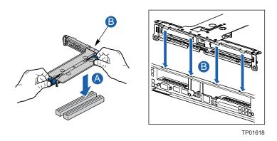
Figure 36. Installing the PCI Riser Assembly into the Chassis
